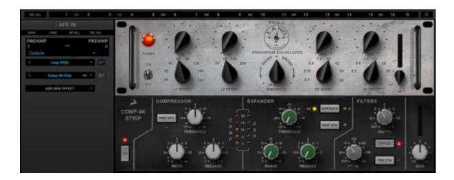
The Effects tab lets you apply up to 8 Synergy Core effects per mono audio channel for a total of 32 channel strips and up to 256 FX instances, independent of sample rate.
