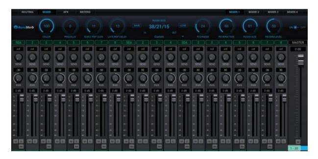
The Mixer tab is home to four 32-channel software mixers. Each channel is equipped with Pan, Volume, Solo, and Link controls (on odd-numbered channels), as well as metering. The Master channel has Volume and Mute controls.
