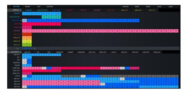
This tab features the Routing Matrix (pictured above) for analog and digital audio routing. The Routing Matrix is row-based. Each row has its own unique color and represents a specific audio in or out with its maximum number of channels.
